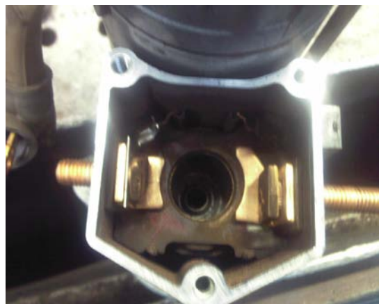
5: Assemble in reverse order NB, the wire goes between head of bolt and contact. Re-use all o'rings / insulators.
